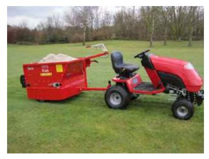
The towed Rink TB950 can be pulled by virtually any vehicle. The weight of the unit is distributed over 4 wheels in order to minimise ground pressure and maintain manoeuvrability. The easy to load hopper handles a range of material which are evenly spread thanks to the adjustable gate & brush.
