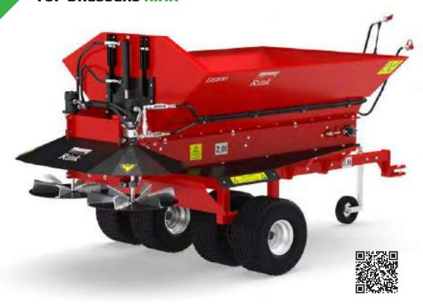
DS800 trailed, this disc spreader has a hopper capacity of 0.8m<sup>3</sup>. The operation of the belt and spinners is carried out from the tractor seat.
