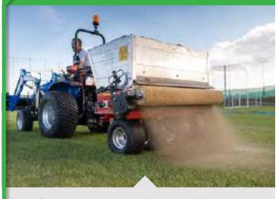
The floatation tyres minimise ground pressure and the lightweight hopper is made of aluminium to avoid corrosion.
