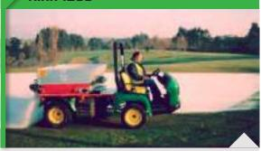
The Rink 1205 hoppers are made of aluminium and can be mounted onto utility vehicles. They cover the tyremarks of the vehicle due to their large working width of 1.8m. Rink 1205 for the John Deere Progator (above).
