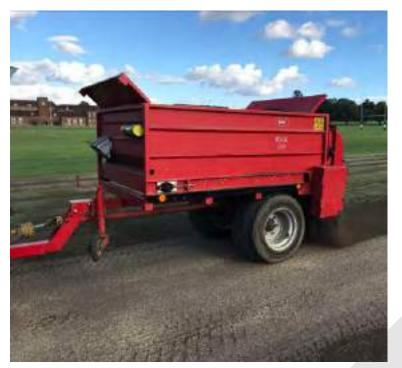
The Rink 2020 Drum spreader is ideal for spreading coarse material, with a tough belt and rear spreading the drum, the 2020 can handle green material with ease. The 140cm (55") working width allows the 2020 to fit in smaller areas such as vineyards and green spaces
