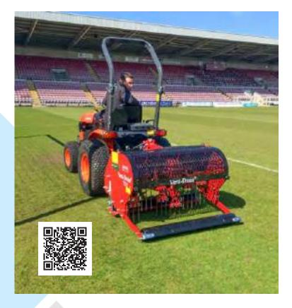
The 72 Series Verti-Drain's® are well suited to lower hp tractors where access is restricted or a lighter footprint is required. These highly productive machines are easily adjusted and work to a maximum depth of 25cm (10") and use 12mm or 19mm (½" or ¾4") tines or mini-tines which are often used for summer aeration.
