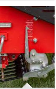
Manual Depth Control gives simple depth adjustment.
