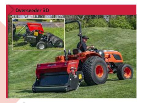
The Overseeder buries the seed up to 20mm(3/4") deep in the ground, safe from the beaks of hungry birds and out of the way of the wind. The amount of seed is controlled to a highly accurate degree and the Overseeder takes undulating ground firmly in its stride. This is thanks to individually mounted coulters that allow the seeder to work in difficult conditions.
