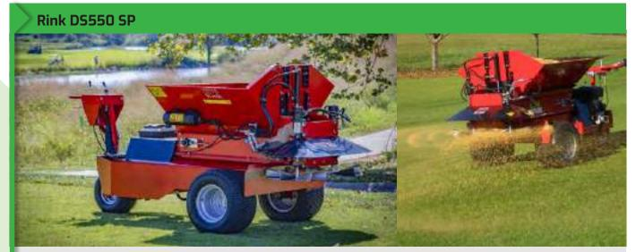
The DS550SP is an ideal tool in areas where manoeuvrability is key, the self-propelled unit is powered by an 18hp engine to ensure maximum performance. The operator can make adjustments while on the move thanks to the easy-to-use controls. The discs will spread material up to 12m (40') with accuracy
