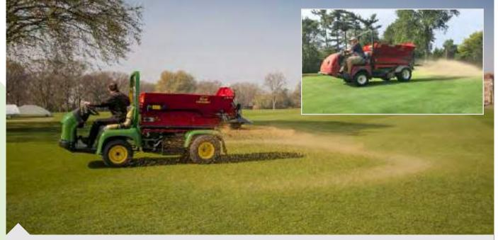
The Rink DS800 can be mounted to either a Toro Workman or John Deere Progator.
