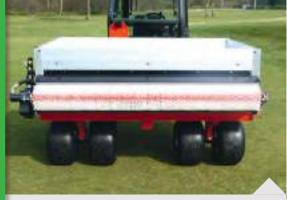
The Rink 1210 has low sides, for easy refilling and ensures the operator has a good rear view.
