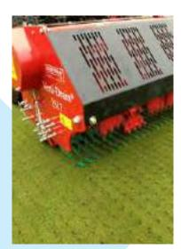
**Optional items** Solid Tines from  $\emptyset$ 5x125mm (3/16"x5") to  $\emptyset$ 12x150mm ( $^{1}$ /2"x6"). Hollow Tines from  $\emptyset$ 10x125mm (3/8"x5") to  $\emptyset$ 18x150mm ( $^{3}$ /4"x6") Turf Hold Down Fingers / Windrow kit / Rear Roller.
