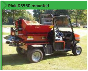
The Rink DS550 disc spreader distributes a range of material, the integrated transport belt moves wet or dry material to the rear of the machine to be spread by the twin discs. The spreading width & thickness can easily be adjusted. The rear door closes to prevent material spillage in transport.
