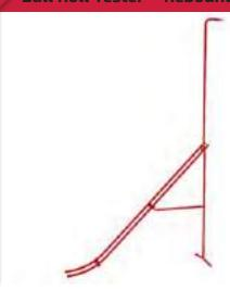
This device measures how far the ball rolls, and how high it bounces and gives an indication on what kind of maintenance is needed.
