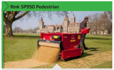
The Rink SP950 is powered by a 6.5hp engine, the weight of the machine is evenly distributed over 6 wheels in order to minimize ground pressure.
