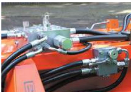
Premium-Hydroblock (optional) und bema SideControl
